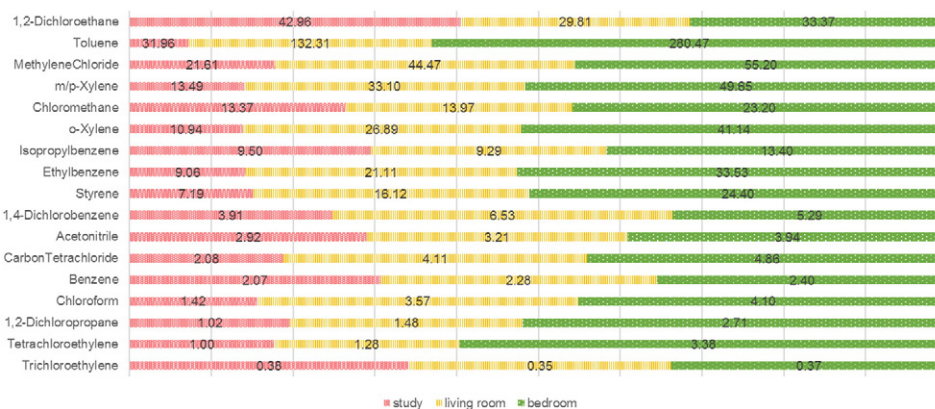
Fig. 5. Percentage accumulation bar plot of indoor levels of target VOCs in different rooms. Data labels indicate mean concentrations (in \mu\text{g}/\text{m}^3 ) of individual VOCs.
